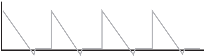
Figure 3: PulseTech Pulse Technology Waveform
